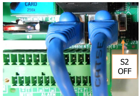
ABB loop-through: S2 OFF (Terminator OFF)
