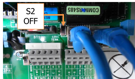
ABB loop-through: S2 OFF (Terminator OFF)
