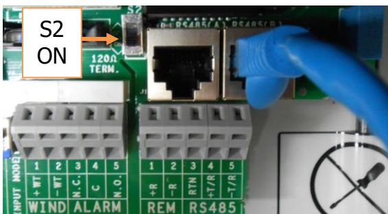
Last ABB on Communications Link (RS485), or when only ABB is used: S2 ON (Terminator ON)
